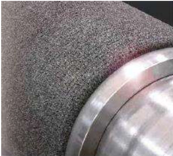
Furnace Roller with brush surface*
