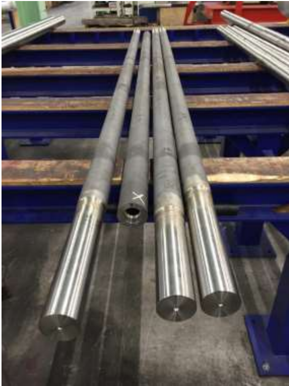
Centrifugally cast shafts before finish machining / welding
