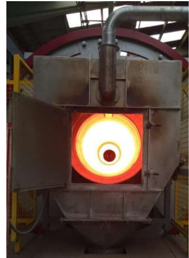
Pre-heated rotary kiln (1150°C)
