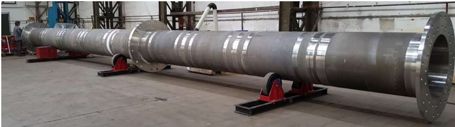
Centrifugally cast rotary kiln drum 9130 x 17.600 mm made in G4879 + 60 HT R with forged flanges
