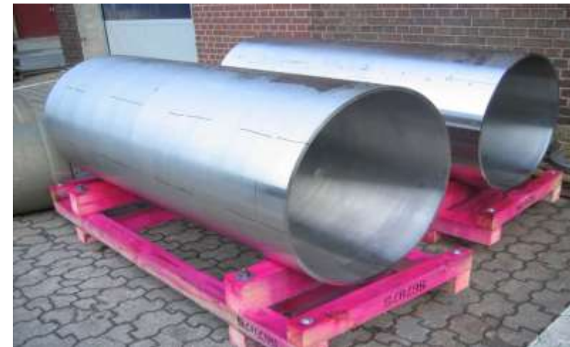
Conductor roller mantles (pre-machined)
