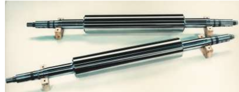
Complete conductor rollers (finish machined)
