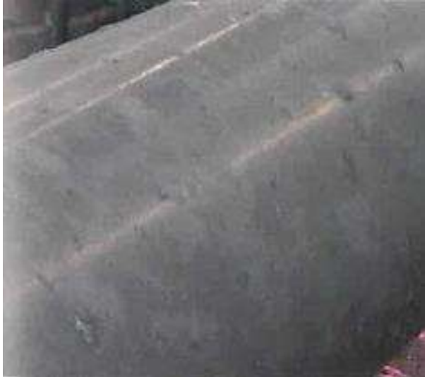
Furnace Roller with pick-up
