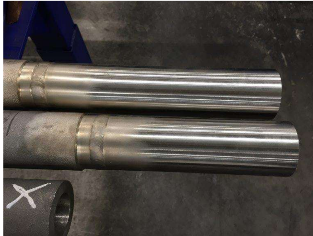
Forged stub ends welded to the castings
