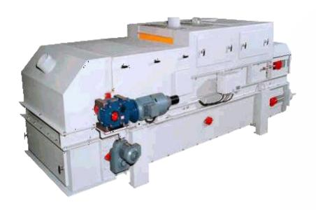
Designed to dose powders such as fly ashes, pozzolana, cement raw meal and any material that has very small grain size and repose angle close to cero
