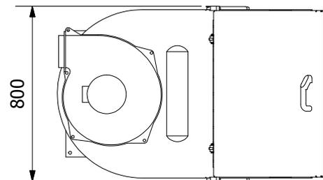
The manual bag dump **Nol-Tec** is a workstation complete with integrated cartridge filters and fan, allowing you to work in a clean and safe environment suitable for use in the chemical, pharmaceutical and food industries.
