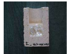
Figure 6: Cup test with soda-lime glass, 96h/1300 °C, University of Pannonia, www.uni-pannon.hu
