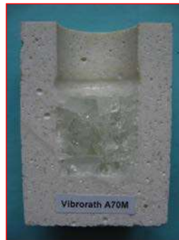
Figure 7: Cup test with soda-lime glass, 96h/1300 °C, University of Pannonia, www.uni-pannon.hu
